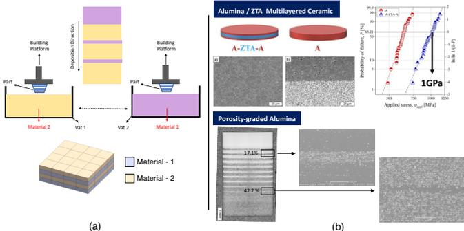
Figure 3. (a) Representation of layer-by-layer approach (b) multi-material samples with heterogeneous and gradient transition zones [7, 8]
