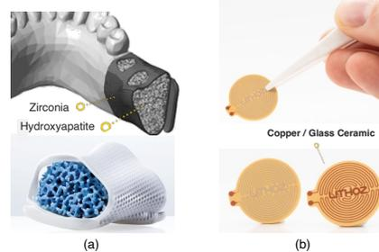
Figure 5. (a) Zirconia/hydroxyapatite ceramic for bone repair and replacement (b) Copper/glass ceramic combination for electronics applications
