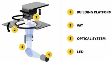
Figure 1. Schematic representation of LCM
