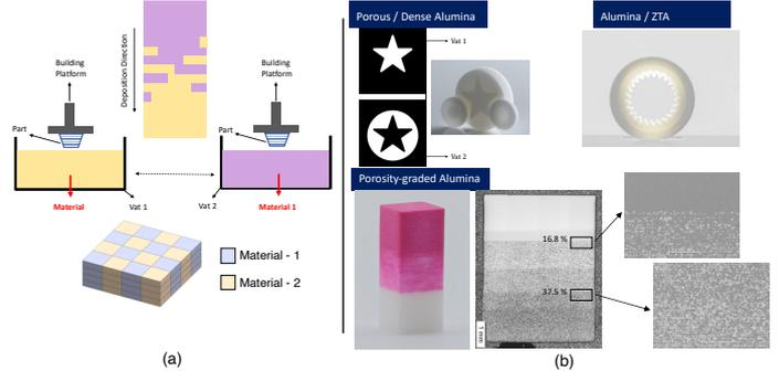
Figure 4. (a) Representation of within-layer approach (b) multi-material samples with heterogeneous and gradient transition zones [8]
